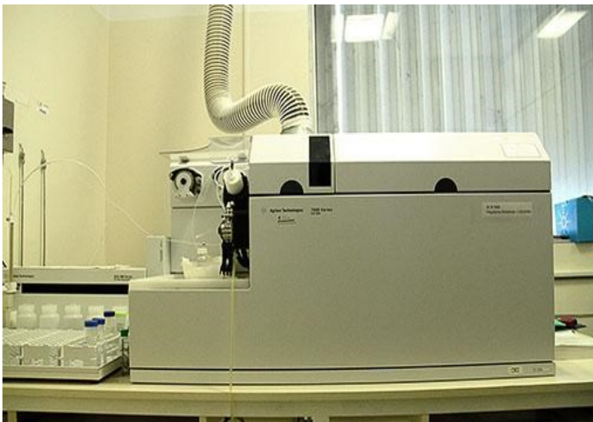
Figure 1. Here is a view of the laboratory, and of the equipment for Inductively Coupled Plasma — Mass Spectrometry (ICP-MS), used in this study.
